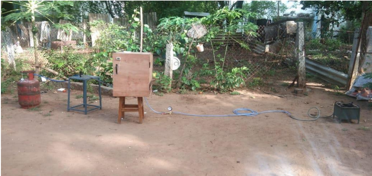
Fig 1.0 Equipment set up of LPG refrigeration system
