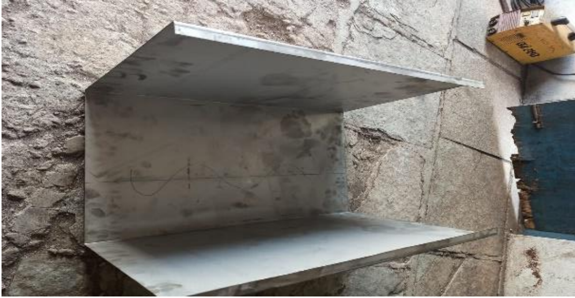
Figure 18 – Bending of SS304 steel.
