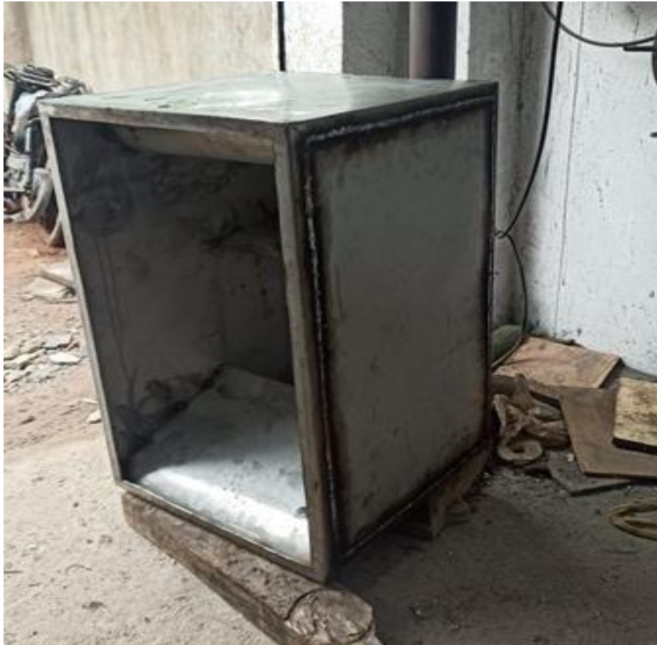
Figure 19 – Assembly after tig welding.
