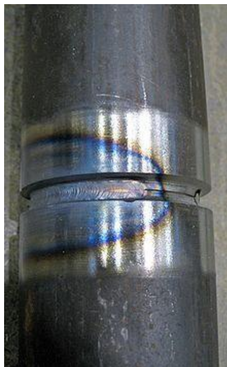
Figure-3 Heat Affected Zone
