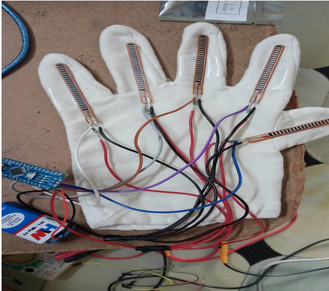
Fig. 20 Construction of Glove
