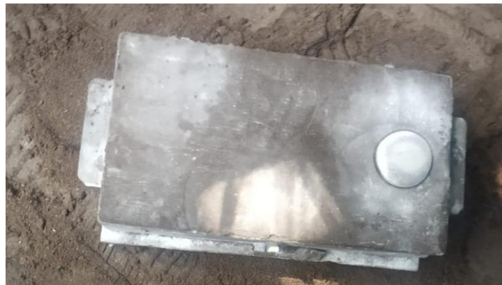
Fig 10: After pouring the molten metal (Filling)
