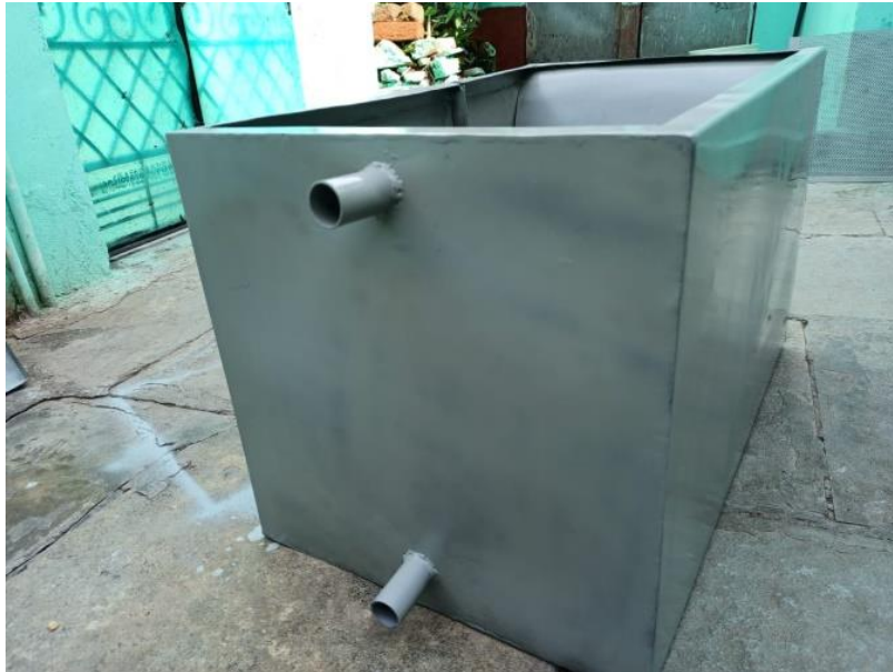
Figure 27 – Final outer shell of the grease trap.
