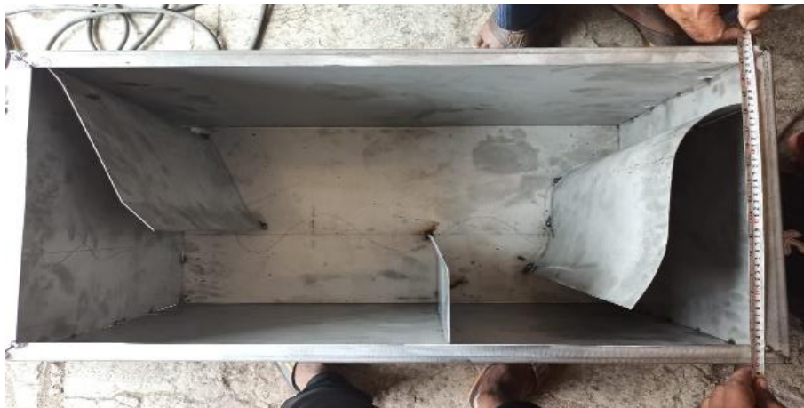
Figure 19 a – Tig welding baffles.
