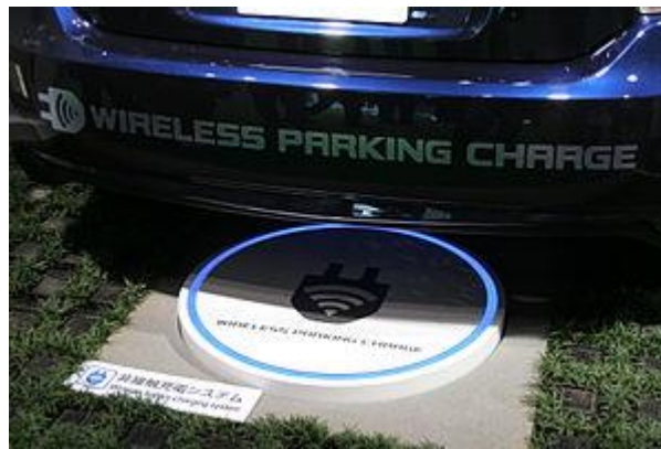
Fig:2.2 Detail of the wireless inductive charging device
