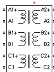
Two winding Transformer
