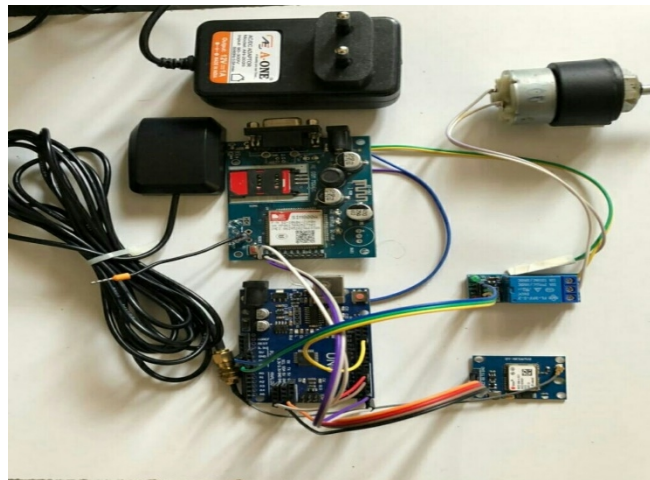
Fig-31: Image of the complete assembly of the different modules of the proposed vehicle tracking system.
