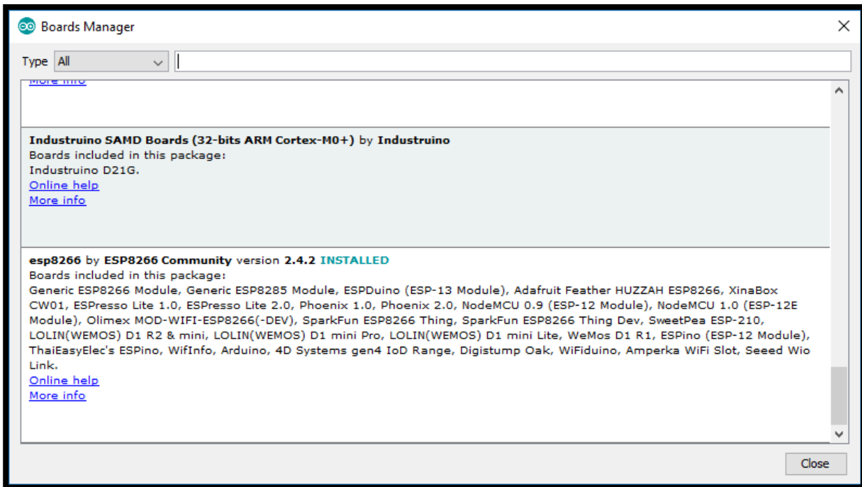
fig 8.7 ESP8266 board is successfully installed for Arduino IDE:
