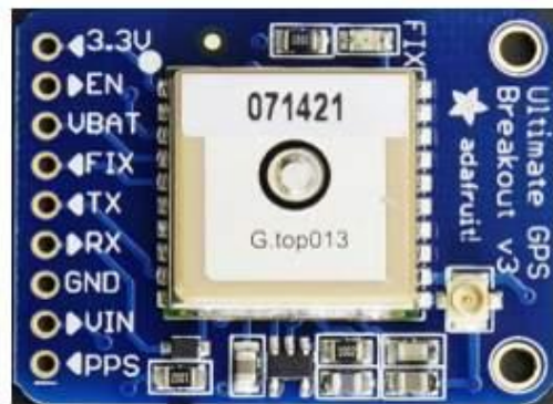
Board with GPS sensor
