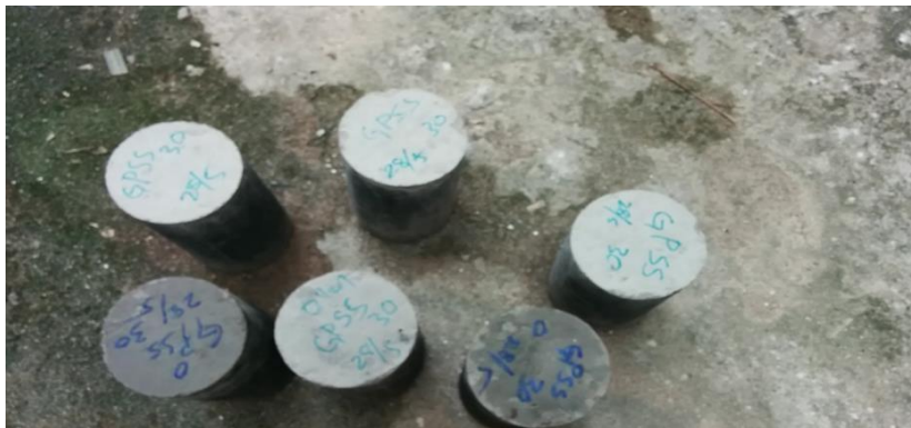
Figure No. 4.3.3 Cylinders after Oven Curing
