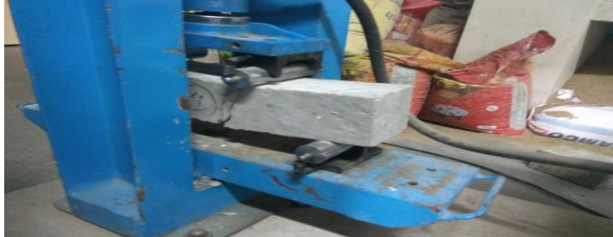
Figure No. 4.4.3 Testing Beam on Flexural strength machine
