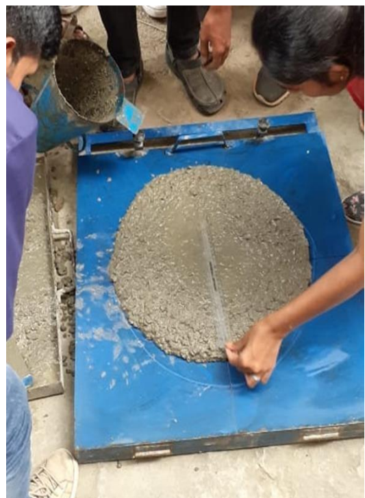
Fig.5 Flow table test
