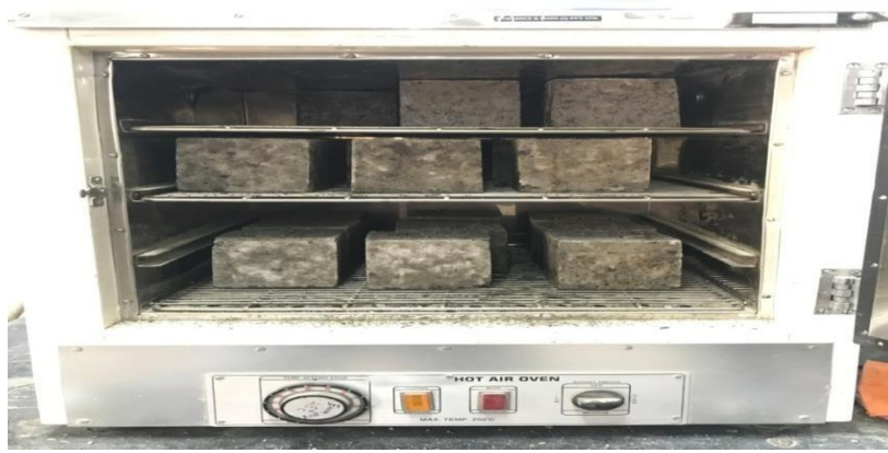
Figure No. 4.3.1 Oven curing of cubes
