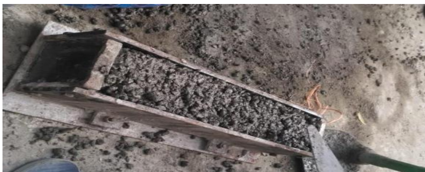
Figure-3.10: casting of prisms
