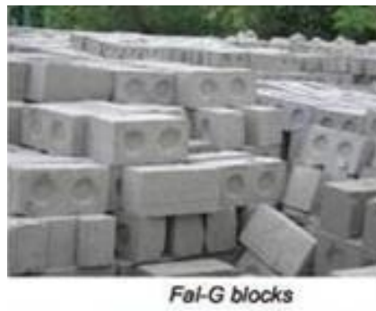
Figure 3.2.4.1 Fal- G bricks
