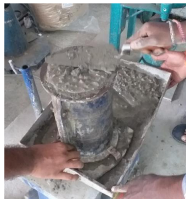
Figure 9: casting of cylinder
