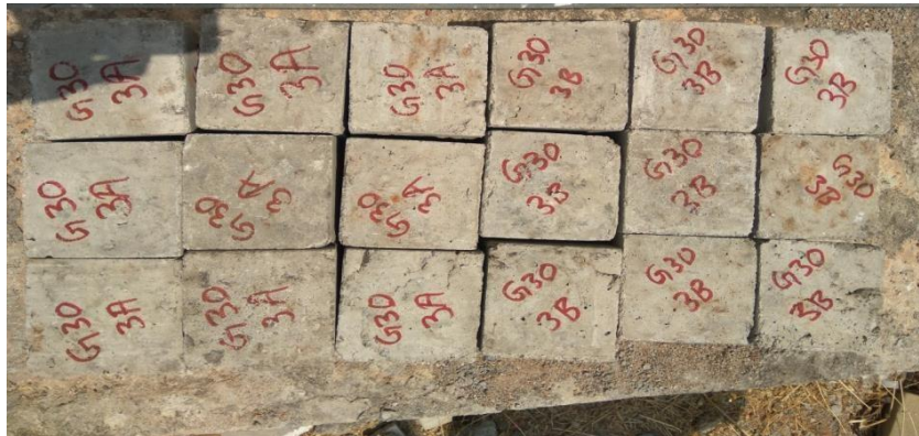
Figure No. 4.3.2 Cubes after oven cured
