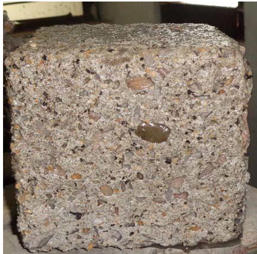
Figure 1.1 Acid attack on concrete
