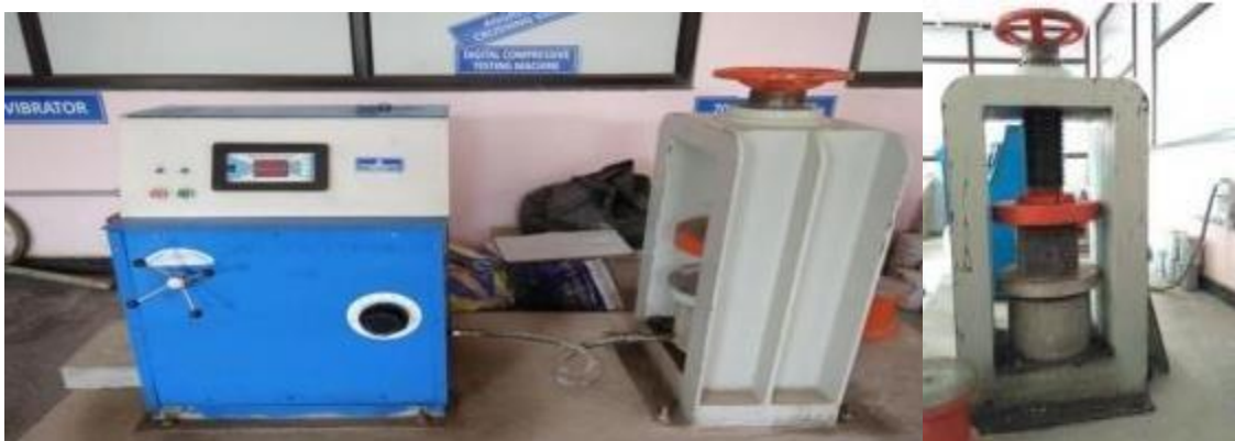
Fig 3-10 Compressive test of cubes
