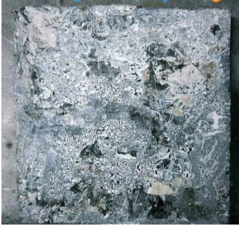
Fig 11: Final LPDE tile
