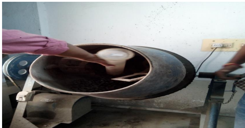
Figure No. 4.1.1 The tilting drum type concrete mixer used for Manufacturing GPC
