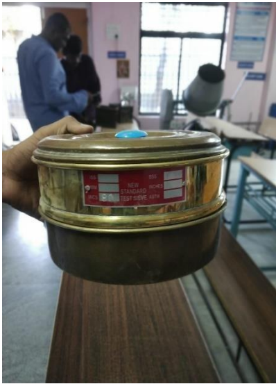
Fig.8 IS: Sieve for fineness test of cement
