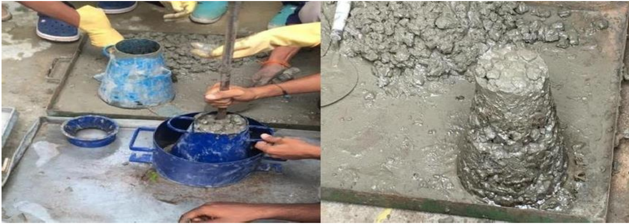
Figure - 3.12: slump testing
