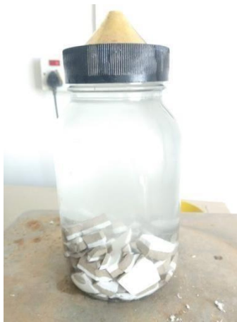
Figure 18: Specific gravity of ceramic waste
