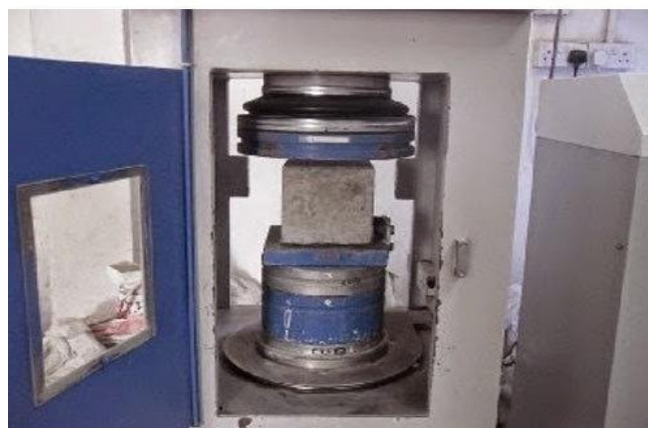
Figure No. 4.4.1 Testing of cubes on Compression testing machine
