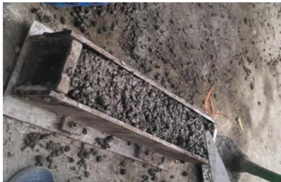
Figure 3.7: Casting of prisms
