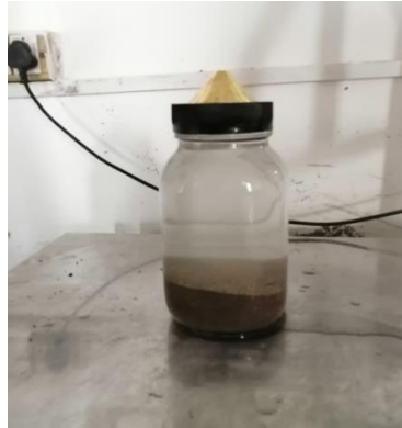
Figure 16: Specific gravity of fine aggregate
