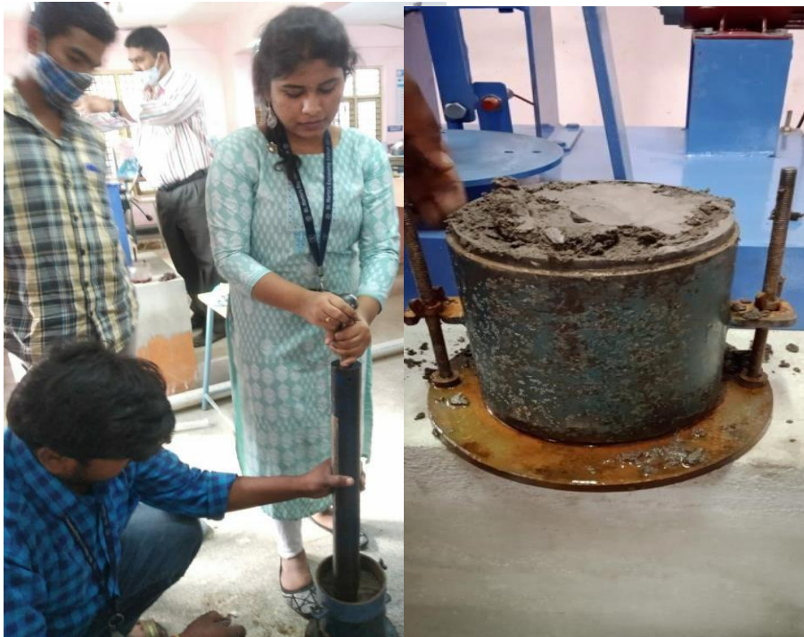
Figure 5.7: CALIFORNIA BEARING RATIO TEST
