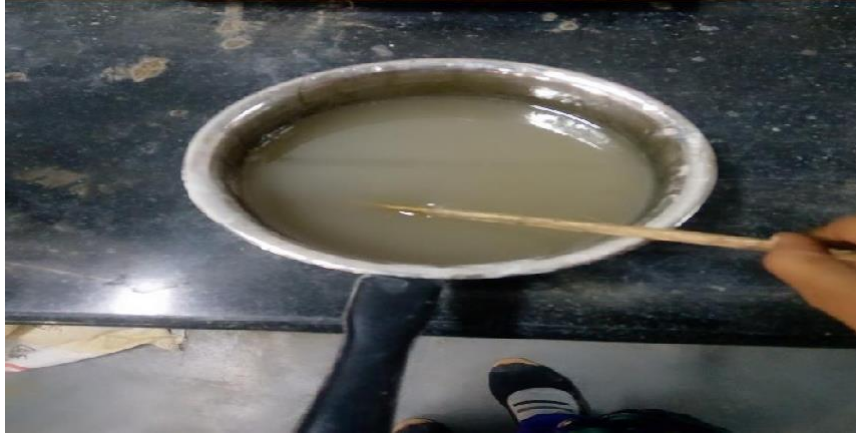
Figure No. 4.1.2 Solution of Sodium hydroxide and Sodium Silicate ( \text{Na}_2\text{SiO}_3 )
