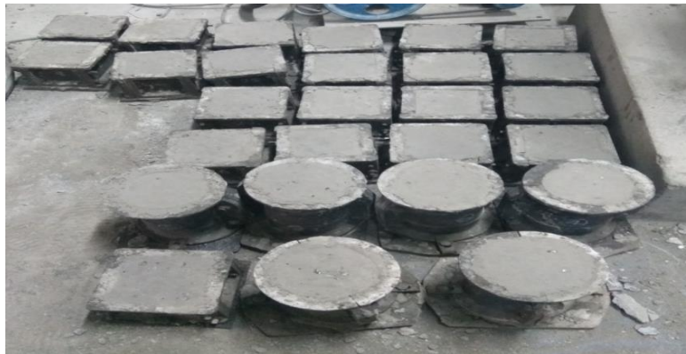
Figure No. 4.2.1 Cubes and Cylinders after casted
