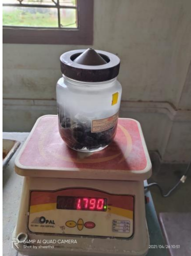
Fig 5.1 specific gravity test for CA
