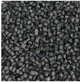
Fig1.2 Black colour nylon compound granules in pellet form
