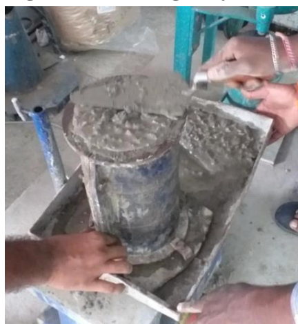
Figure-3.9: casting of cylinder
