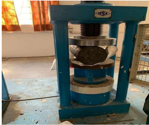
Fig 15: Split tensile test on cylinders
