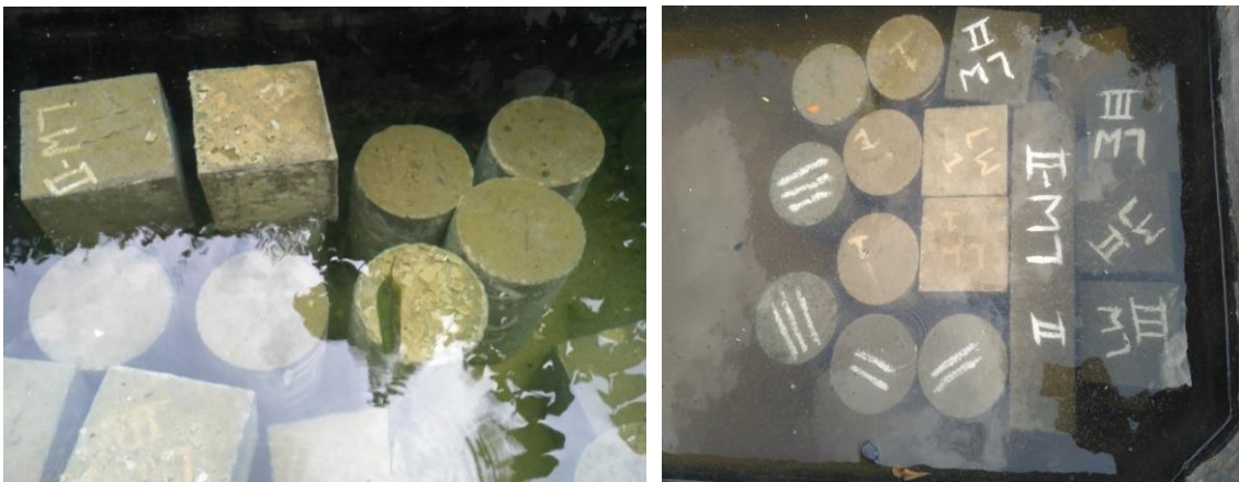
Figure - 3.11: Curing of Specimen.
