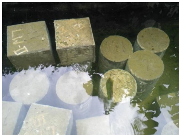
Figure - 3.8: Curing of Specimen.
