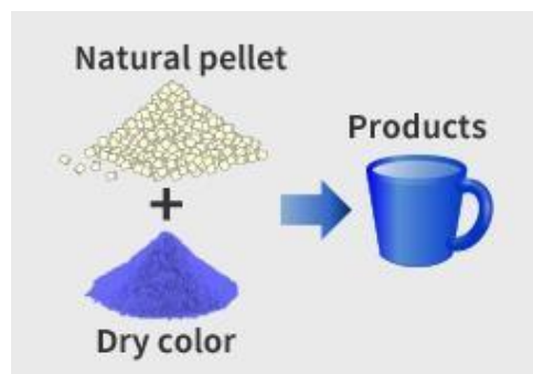
Fig 1.3 Plastic products formed by dry plastic colorants
