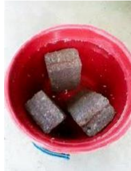
Figure 5.2 water absorption test
