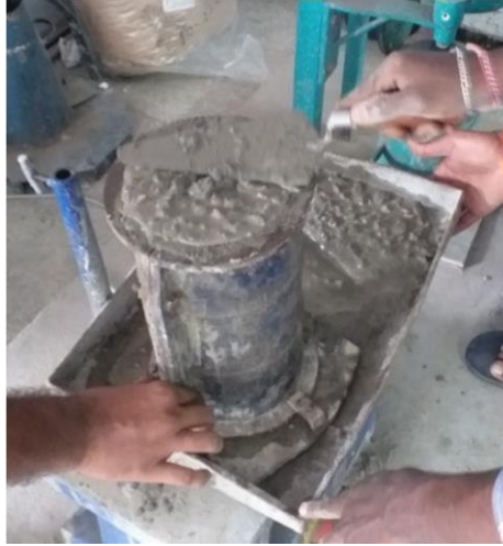
Figure-3.6: casting of cylinder
