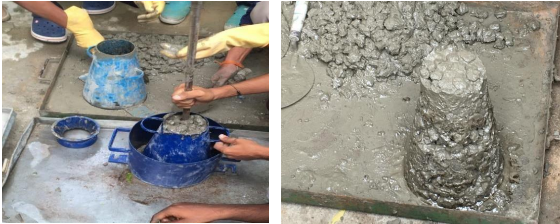
Figure - 3.9: Slump testing
