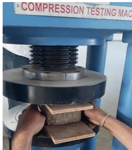
Figure 5.3 Compression strength test
