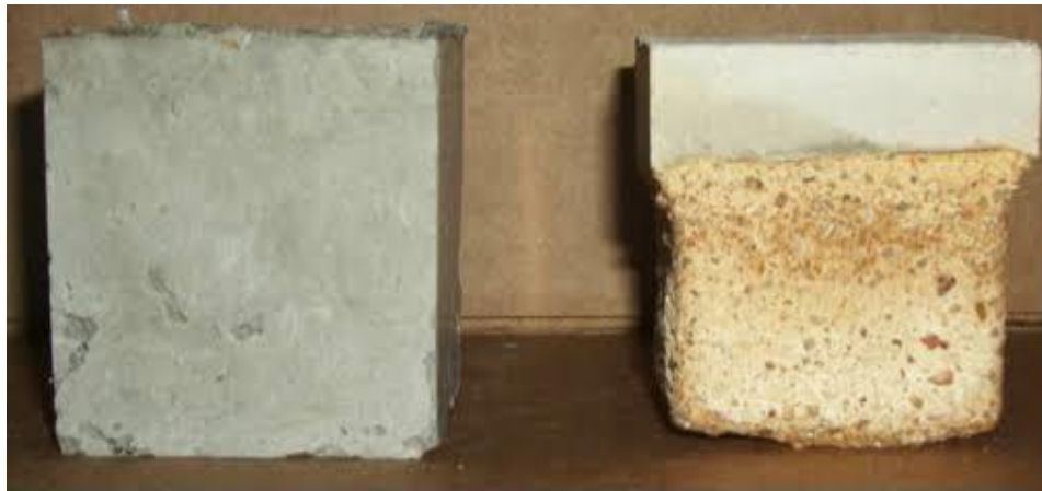
Figure 1.2 Decomposition of concrete
