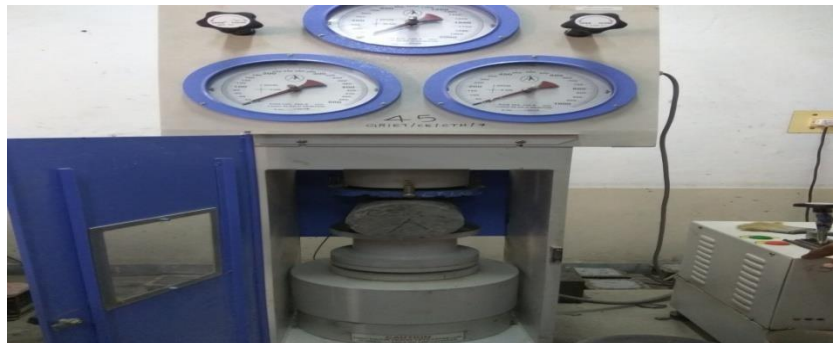
Figure No. 4.4.2 Testing of cylinders on Compressive testing machine
