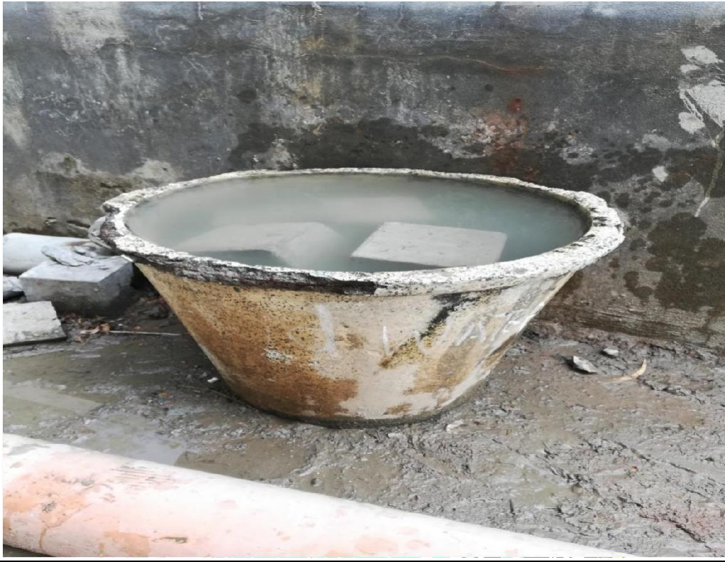
Figure 5.14 HNO 3 solution curing tank.
