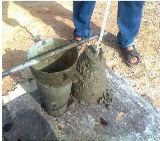
Figure 3-9: Determination of slump as per BS 1881-102 (1983)
