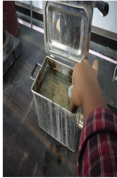
Fig.7 Soundness test on cement
