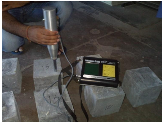
Fig. 3.8 Rebound Hammer Test
