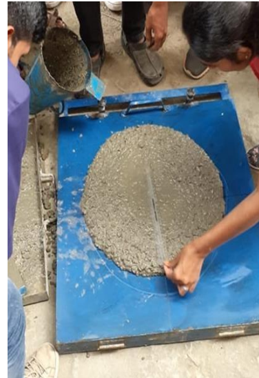
Fig.5 Flow table test
